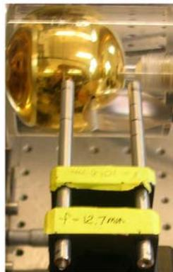
Fig. 2. Photograph of the optical cavity (back) and the collimating lenses for the QC laser (front). The cavity is made from a hollow acrylic body coated inside with gold. Refraction in the acrylic makes the cavity appear more spherical than it is in reality.
